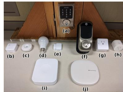
Figure 8: The commercial Zigbee devices that we studied.
